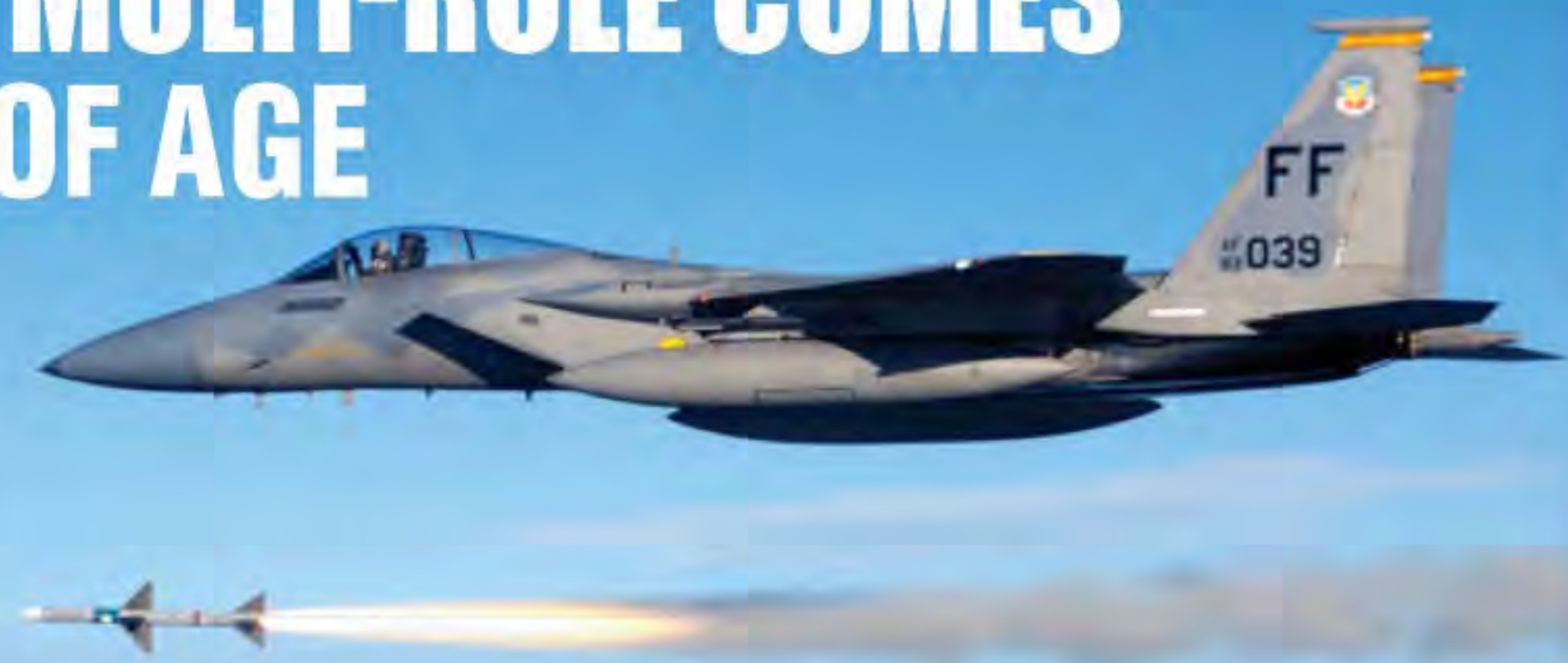
The third-generation F-15 Eagle firing an AIM-7 Sparrow medium-range air-to-air missile during a Combat Archer air-to-air weapons system evaluation program mission United States Air Force. Master Sgt. Michael Ammons
